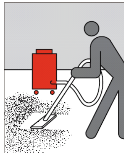
Figure 9: Dusts removed by aspiration Source: Suva
